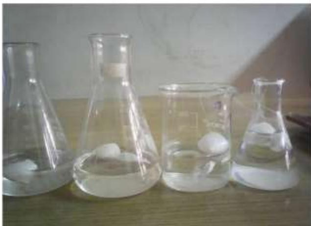
**Figure 2.** Membrane along with the contents suspended in 0.1M Tris buffer
