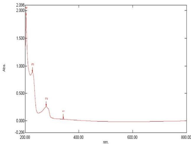
**Figure 2.** UV visible spectrum of PHA produced from *B. subtilis* AMN1. The peak at 230-240 nm confirms the presence of ester group in the polymer
