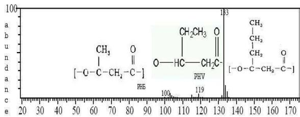
**Figure 6.** Carbon NMR ( $C^{13}$  NMR) spectra of PHA produced from *B. subtilis* AMN1. The peaks indicate the presence of methyl, methylene, and carbonyl groups in the polymer.
