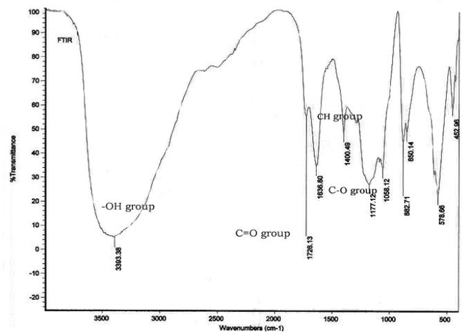
**Figure 3.** FTIR spectra of PHA produced from *B. subtilis* AMN1 indicates the presence of several functional groups in the polymer.
